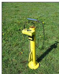
The 2.25Kg Clegg Impact Soil Tester
