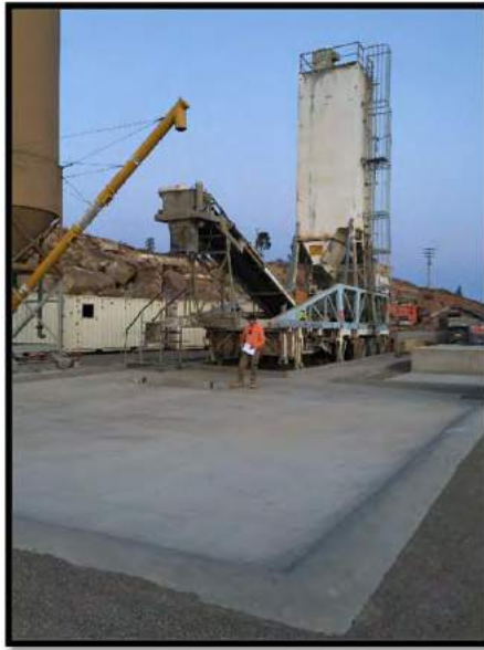
Photograph 23: Mobile Cement Batching Plant. Note the Concrete Walled Area to catch any spillage.
