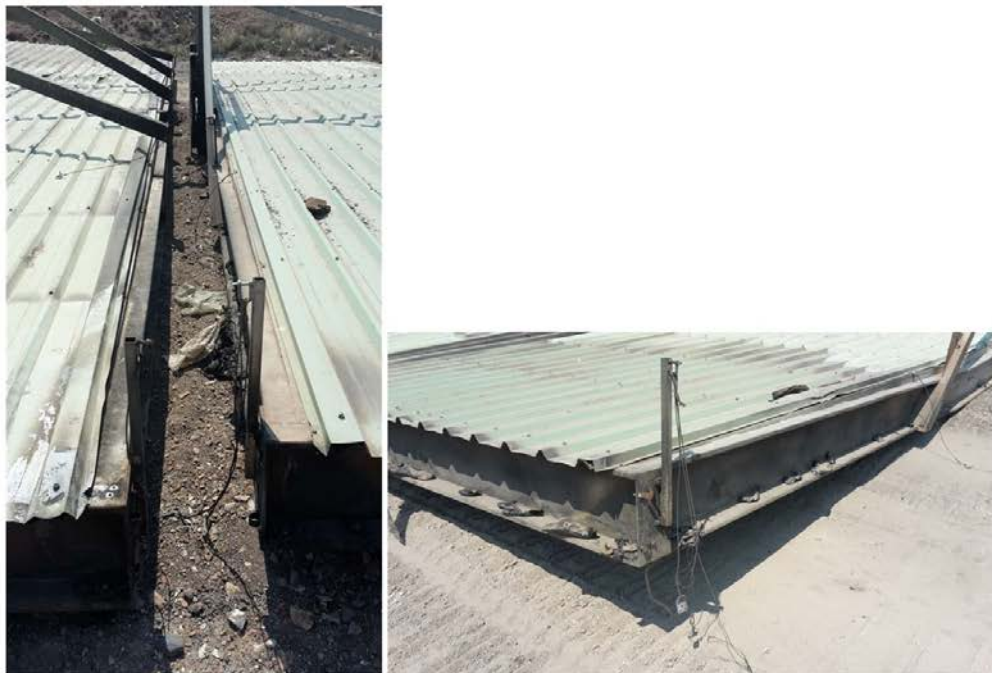
Figure 11: Lid 6 (left) and lid 5 (right) showing complete destruction of rubber skirt assembly and charring of steel and galvanised portions.
