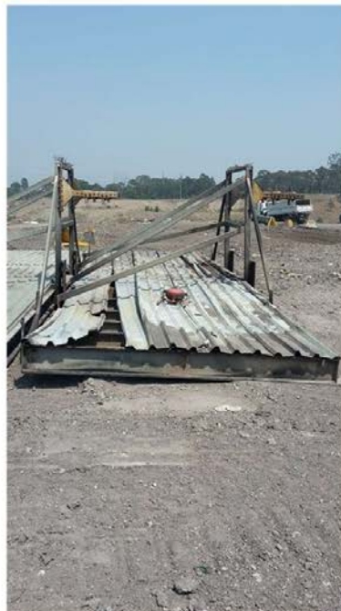
Figure 5: Lid 3. Charring of paint and galvanising evident. Skirts burnt away.
