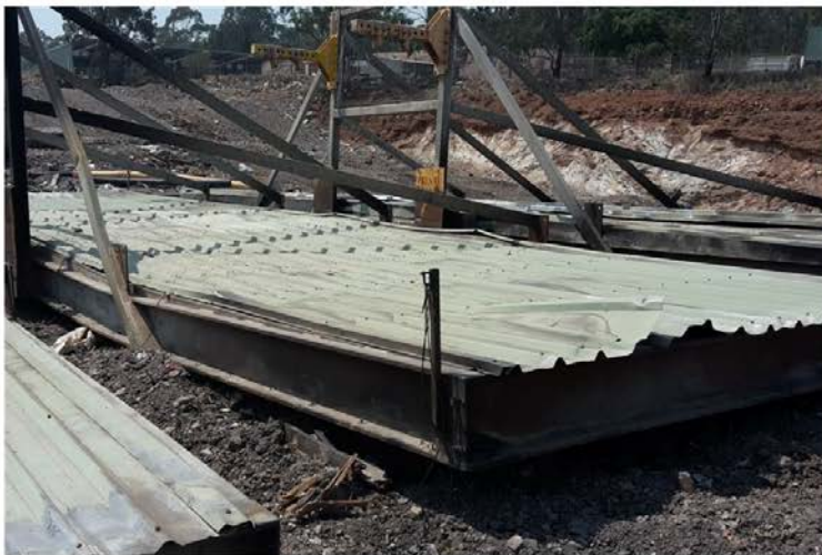
Figure 4: Lid 2, charred and warped, skirting destroyed.
