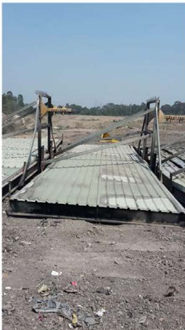
Figure 5: Lid 3. Charring of paint and galvanising evident. Skirts burnt away.
