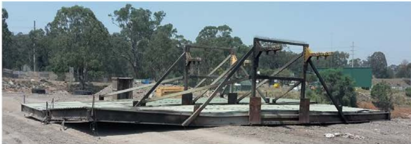
Figure 8: Lids 5 and 6. Lid 6 (in foreground) showing charring and warping.
