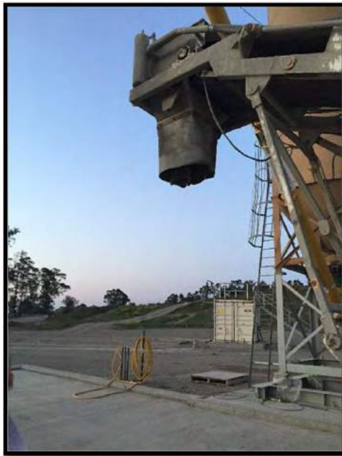
Photograph 26: Close up view of the Mobile Cement Batching Plant and operation all taking place above the Concrete Walled Area to catch any spillage.
