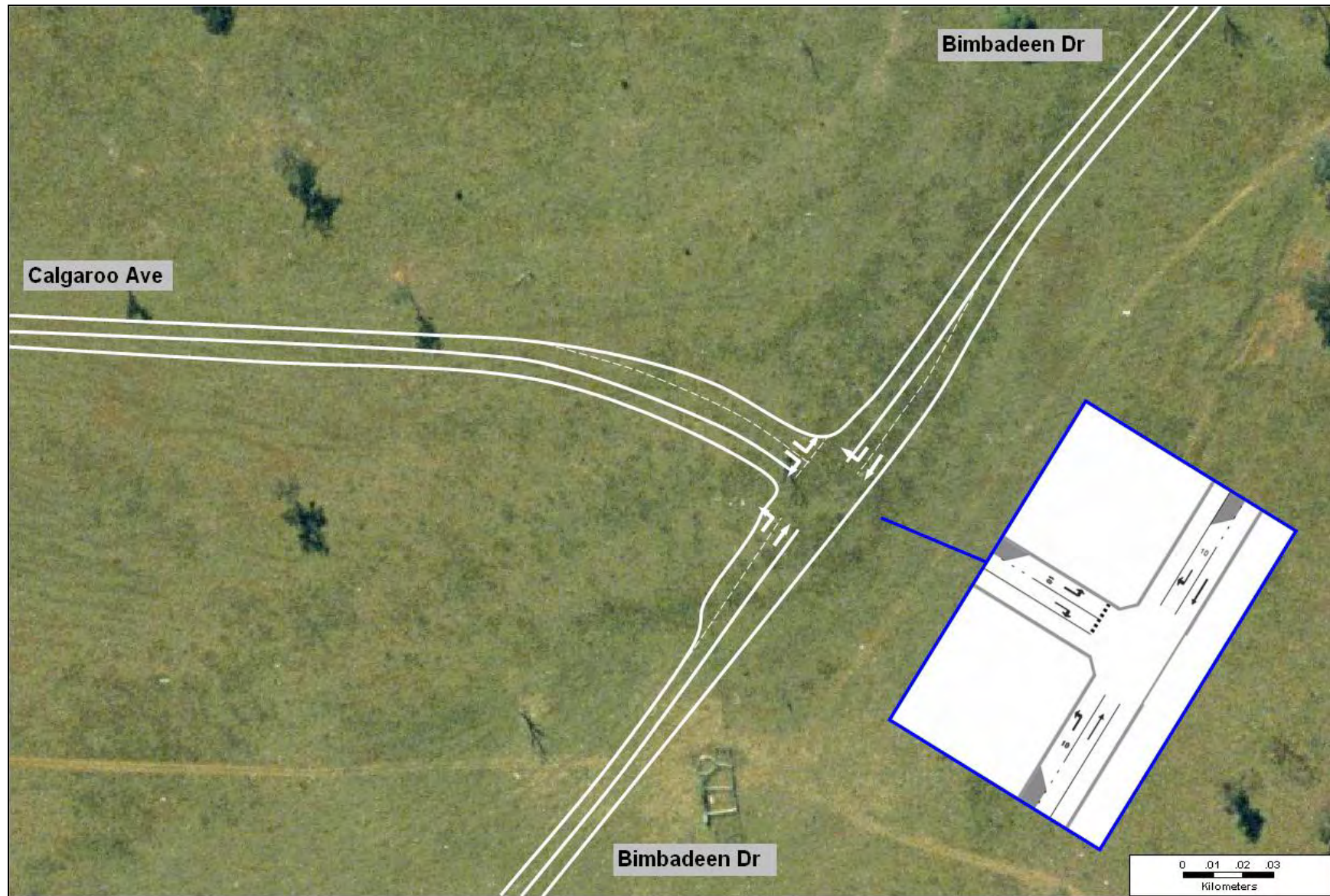
Figure 8-16 New intersection at Bimbadeen Dr/Calgaroo Ave (with auxiliary lanes-type B)
