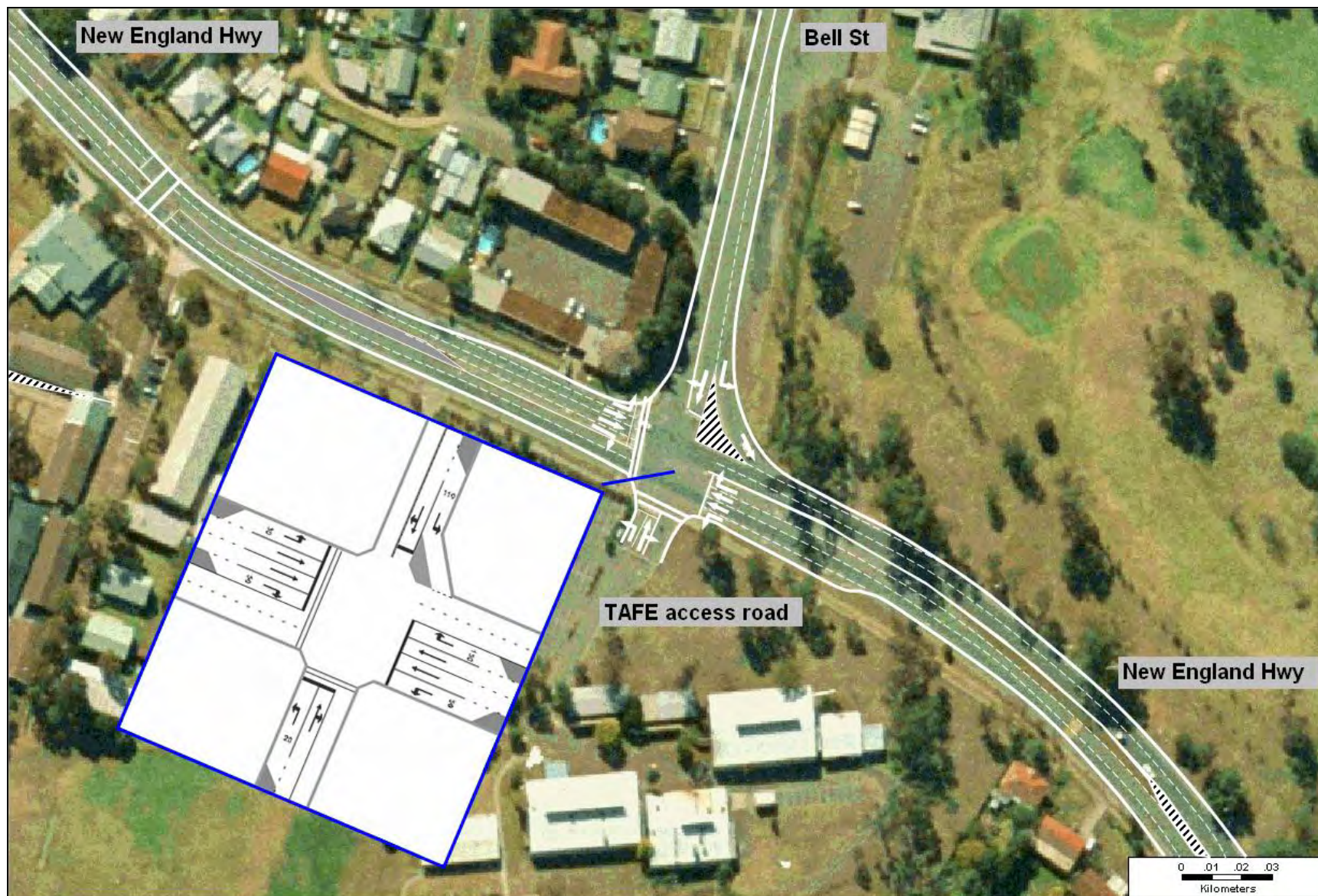
Figure 8-9 Intersection upgrade at New England Hwy/Bell Street (by extending the length of turn bays)
