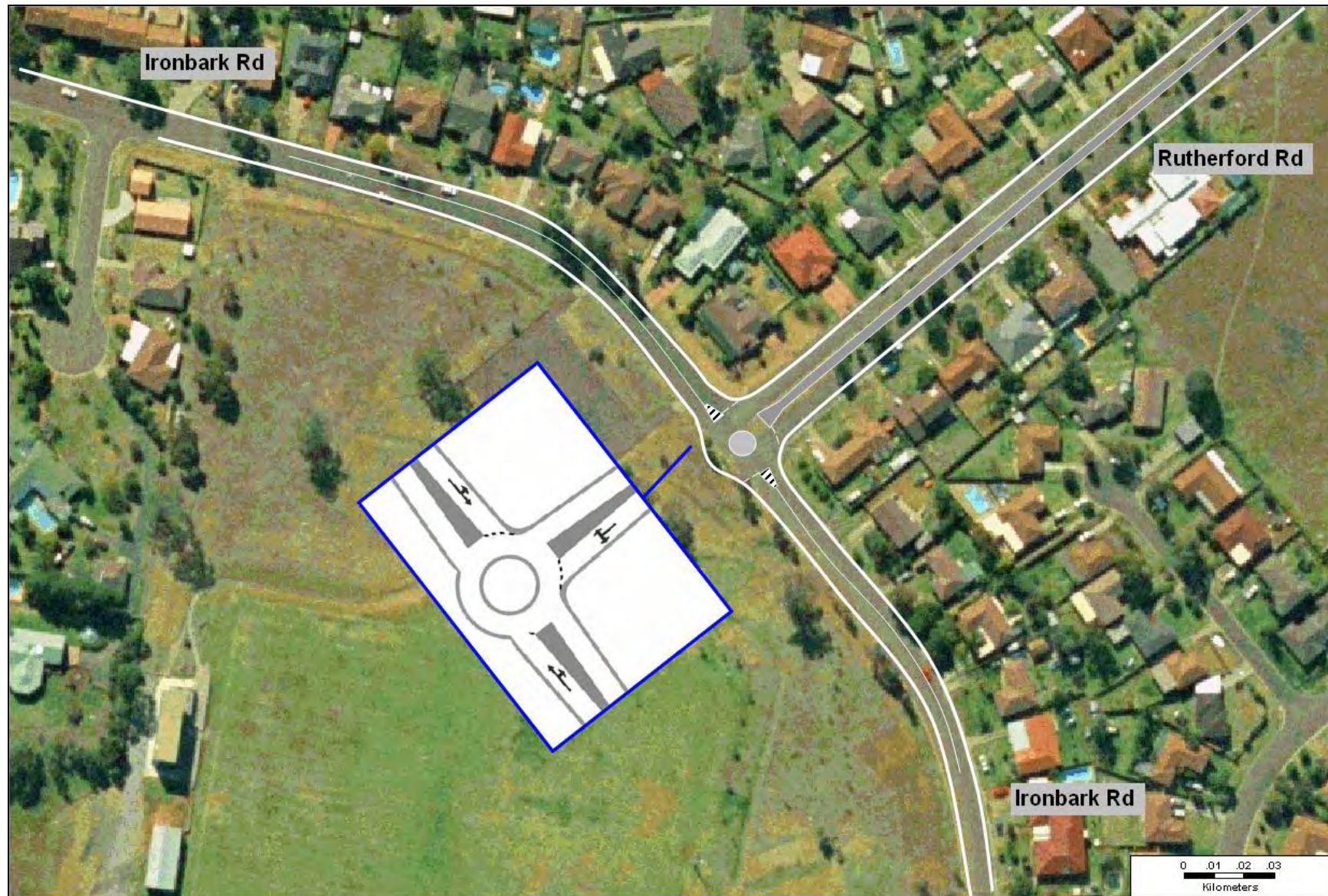
Figure 8-3 New single-lane roundabout at Rutherford Rd/Ironbark Rd
