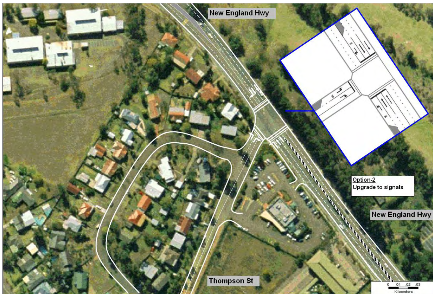
Figure 8-5 New signal at New England Hwy/Thompson Rd (Option-2)
