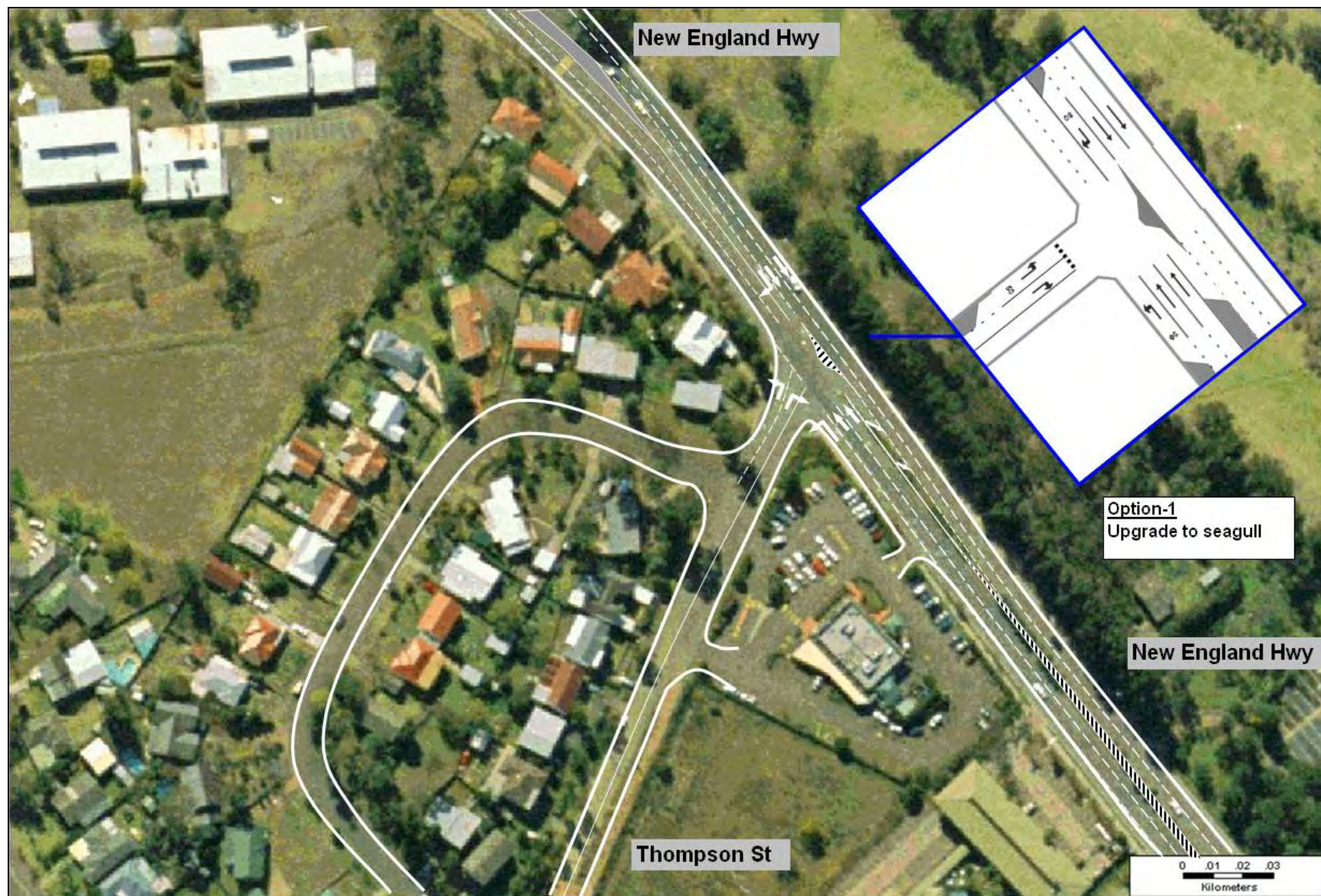
Figure 8-4 Seagull type arrangement at New England Hwy/Thompson Rd (Option-1)
