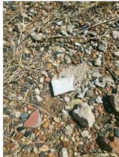
Photo 4. Positive ACM fibre-cement fragment found in the north-western portion of the Site.
