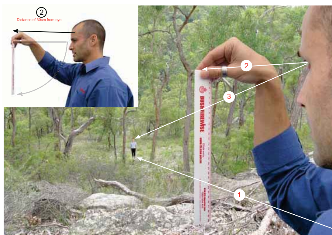
Fig 4. Simple slope assessment methodology.
