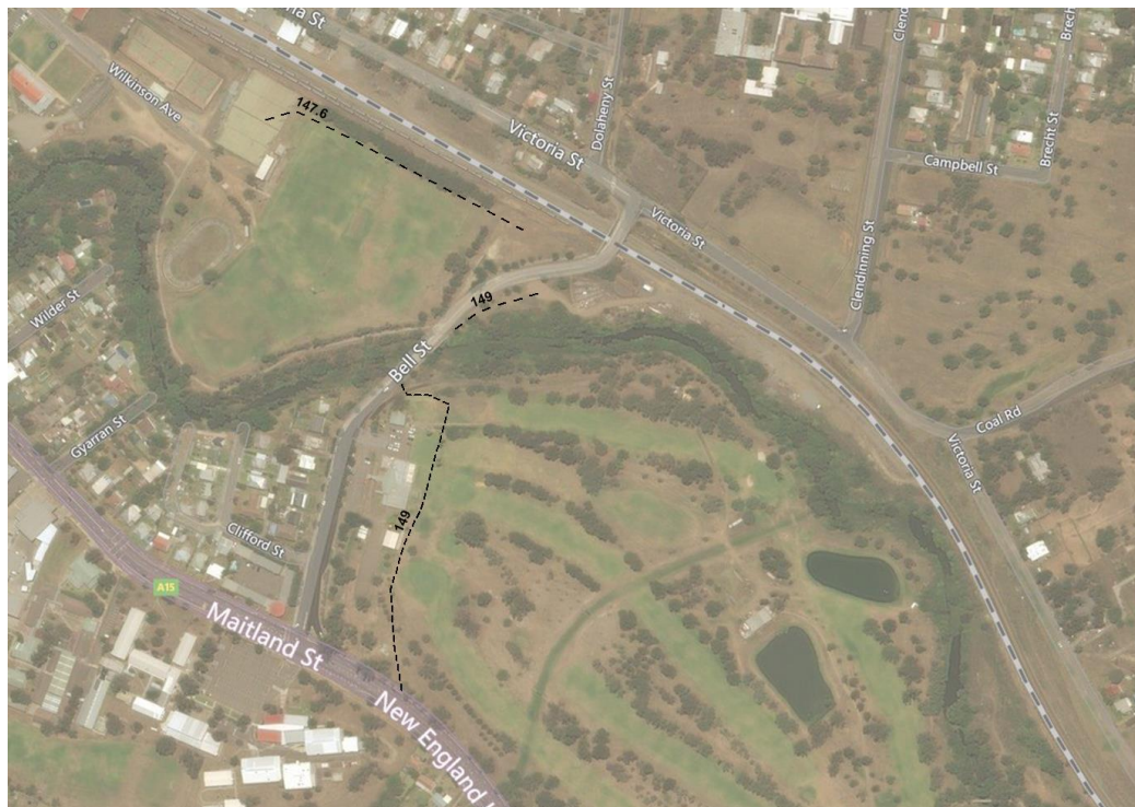
Figure 6-6: Outline Details of MC2 – Muswellbrook Golf Course Flood Bund
