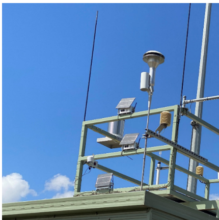
Clarity air sensors deployed at the Bowman Park Air Quality Station for calibration.
