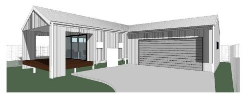
View of Granny flat and garage. Simple galvanised steel building that is modern but offers traditional forms that will assist in blending into the context. It is a similar height bulk and scale as surrounding buildings.
