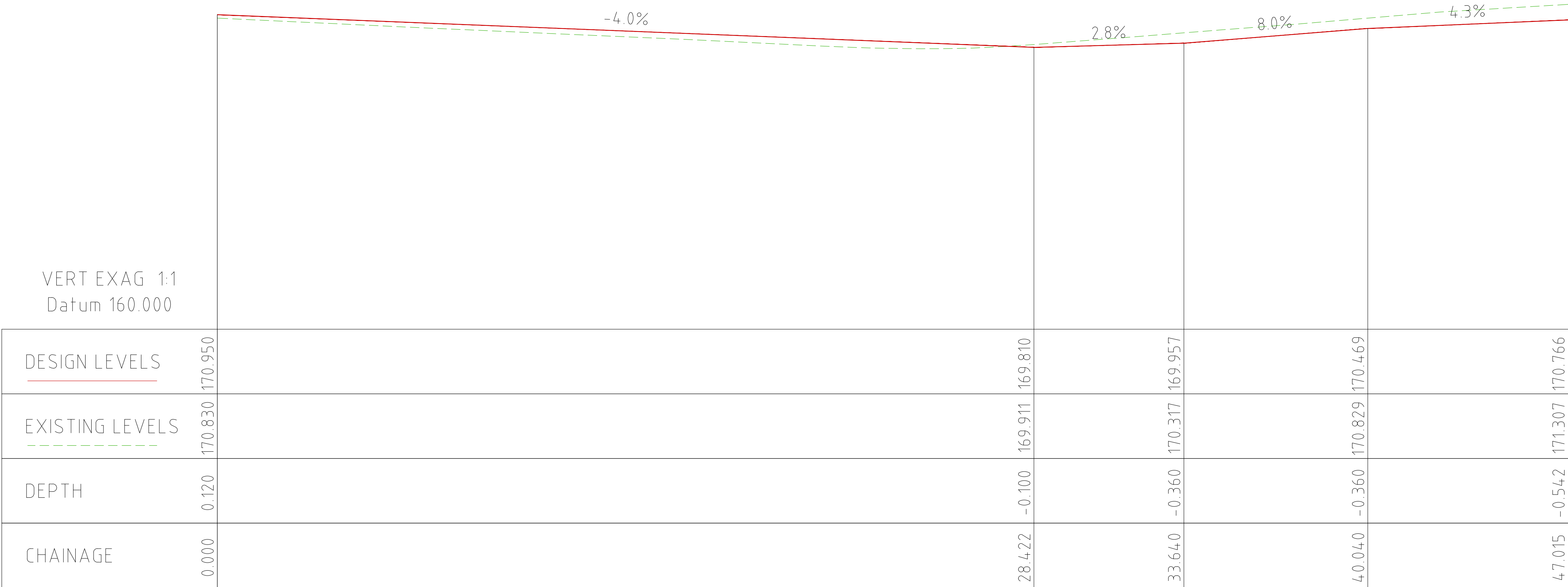
ROAD 02 LONGITUDINAL SECTION 1:100 @ A0 (H & V)
