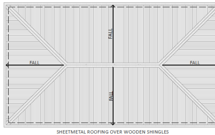
02 PLAN - ROOF EXISTING WORKS
