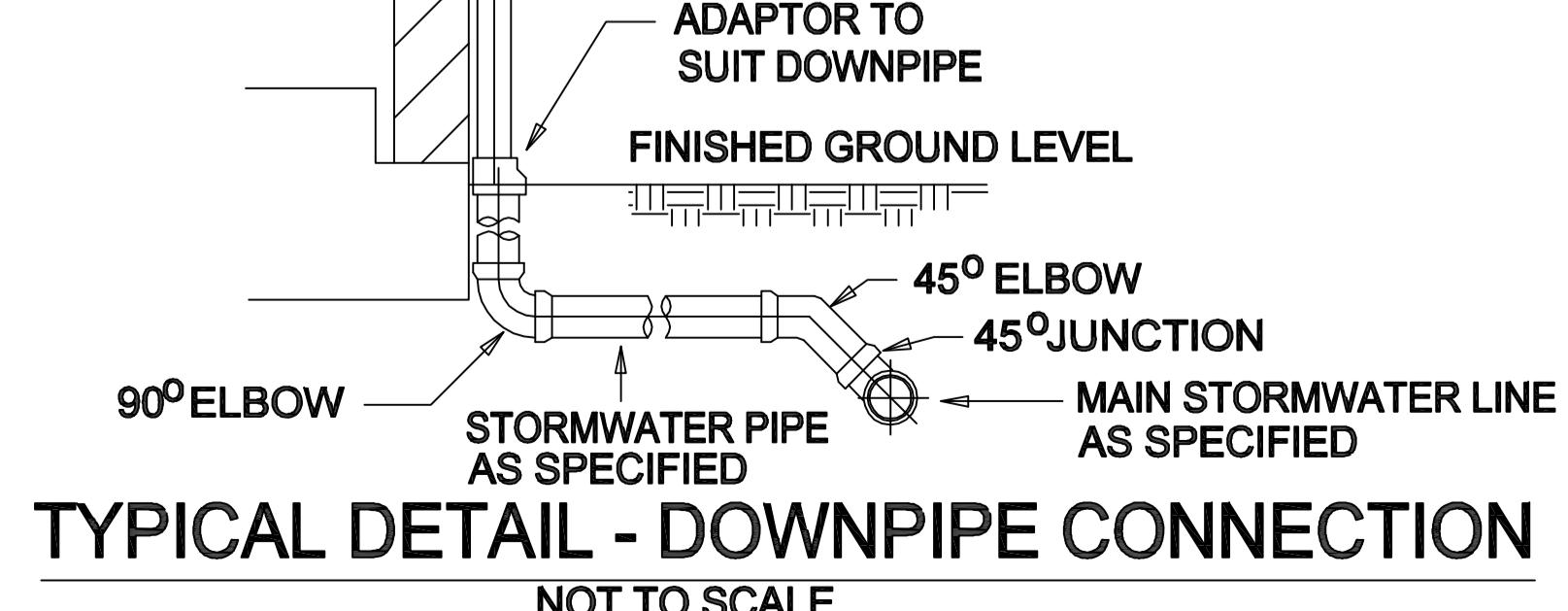
**TYPICAL DETAIL - DOWNPipe CONNECTION**
