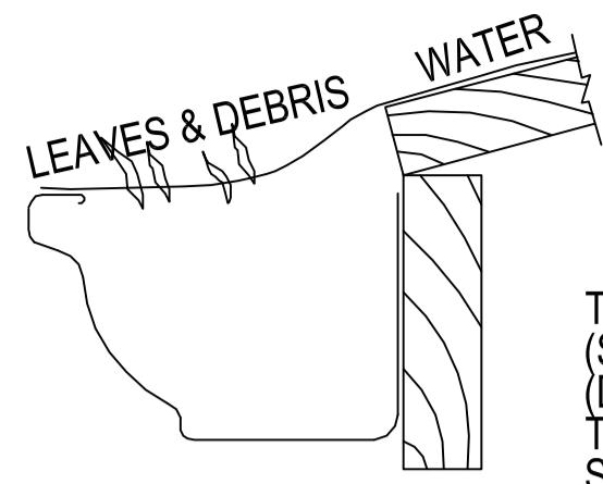
**TYPICAL DETAIL OF GUTTER PROTECTION**
