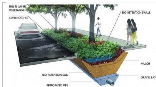
Figure 2-19: Bioswale concept diagram (Brankovic, n.d.)
