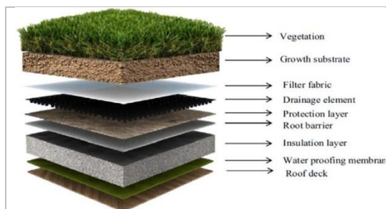
Figure 2-21: Green roof components (Khawaja, 2018)
