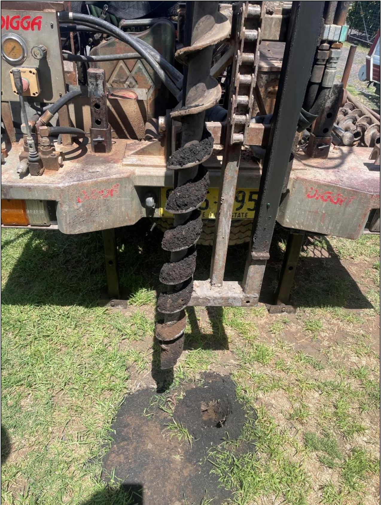
Figure C7: Fill materials, consisting of imported coal-wash, encountered within BH01 and BH04
