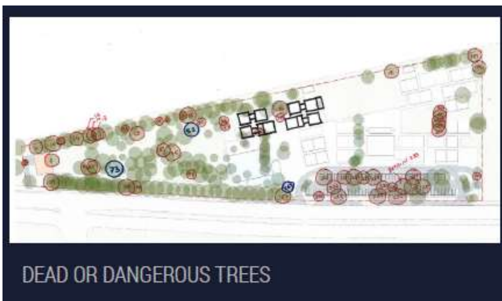
Figure 7 NBRS Markup of dead and dangerous trees
