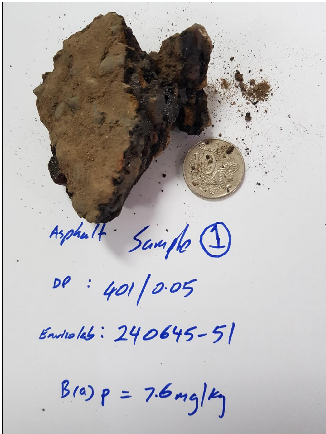
Figure 35: Photo of surface asphalt from test pit 401.
