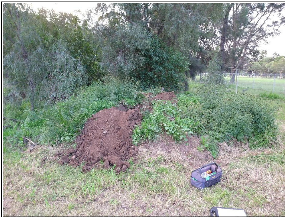
Figure 13: Stockpile 306 located in the central northern portion of the site, generally comprising silty sand and gravel and intermixed clay with trace asphalt.
