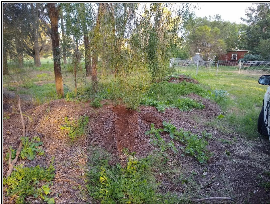
Figure 14: Stockpile 307 located in the western portion of the site, generally comprising silty sand and gravel.
