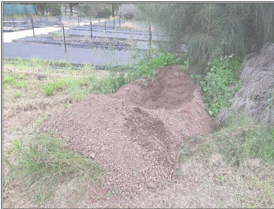
Figure 11: Stockpile 304 located in the central northern portion of the site, generally comprising silty sand and gravel.
