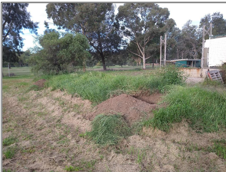
Figure 10: Stockpile 303 located in the central northern portion of the site, generally comprising silty sand and gravel.
