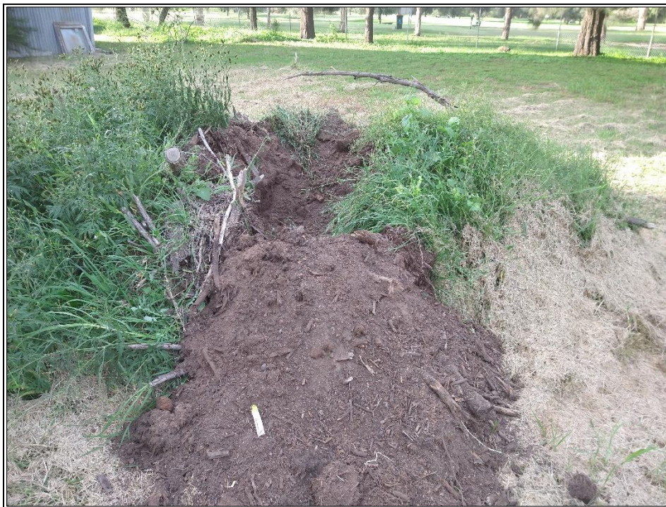
Figure 7: Stockpile 301A located in the eastern portion of the site, generally comprising gravelly silty sand and abundant vegetation.
