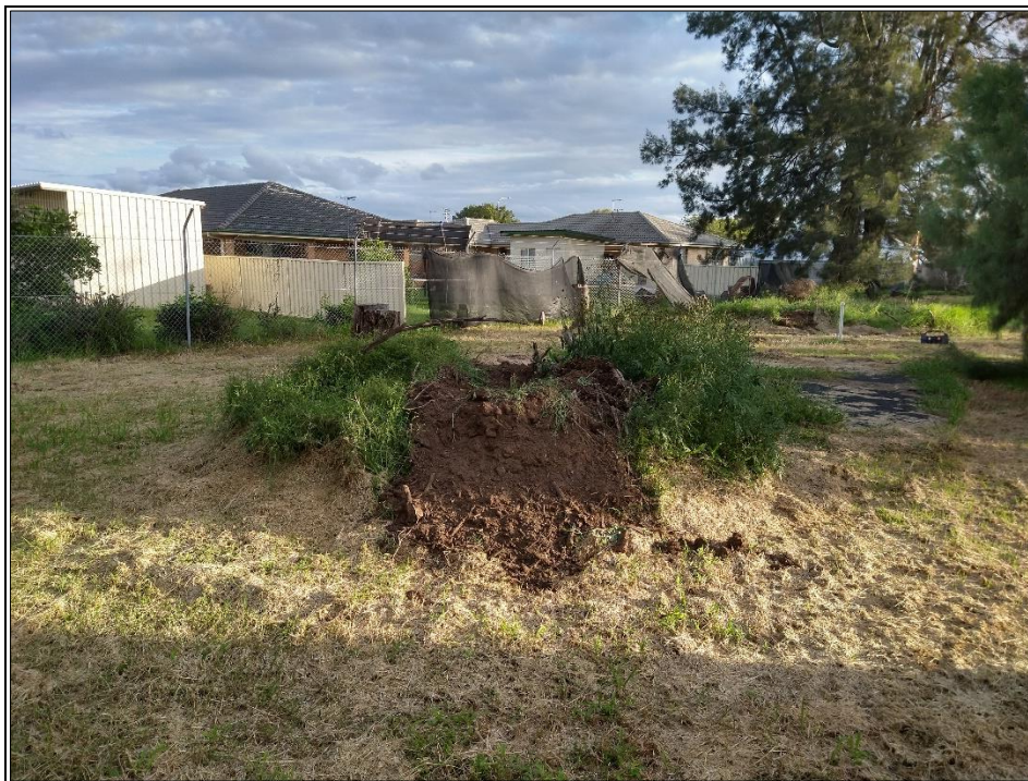
Figure 6: Stockpile 301 located in the eastern portion of the site, generally comprising gravelly silty sand and abundant vegetation.
