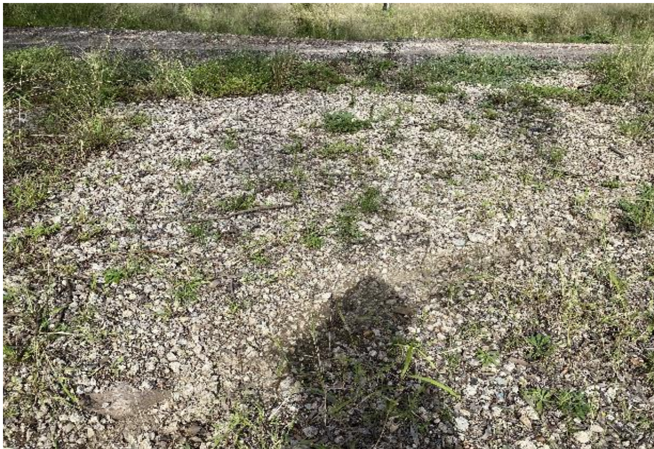
Photograph 13 - Showing thin layer of concrete rubble.
