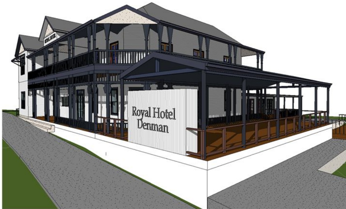
Figure 02 – View of the new roofed deck area and freestanding Screen unit. The subfloor of the existing deck is continued down Ogilvie Street frontage and rendered, this then extends around enclosing the subfloor, creating a cohesive and quality appearance. The freestanding screen unit is an attractive design element with vertical fc Vj board. The proposed signage with led lights provides a quality appearance to the street. The new roof integrates with the existing steel poles on site and does not dominate the existing Hotel Building. Everything integrates simply and elegantly.
